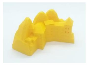
To print the Predjama Castle, we have scaled the original Tinkercad model until get a size of X:70,50 Y:53 Z: 40,09, because when we added the back cave, the design increases its size hampering the time and 3d print process.
