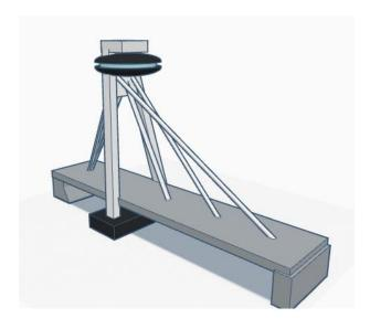
It is a structure with some difficulties when we have to print it, the main problem is the material printed in the air for a long time (it depends on the scale), this problem is known as bridging.
