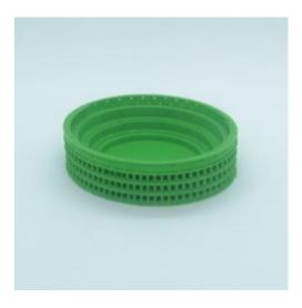
The printing problems of this design will depend, basically, on which scale we are going to print it. These problems will arise at colosseum arches print, considering that if we print it on a large scale, we could have "Bridging" problems.
