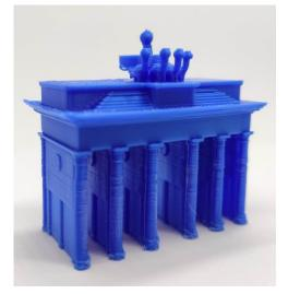
This model is not hard to print, the only difficulty could be the "stringing" between the gate pillars, but it is easily removed on post-processing step.
